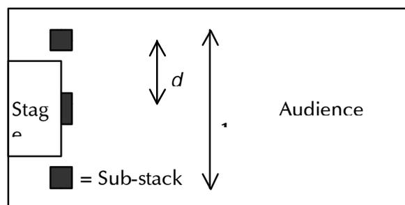
Fig.1 typical sub-stack layout (topview).
