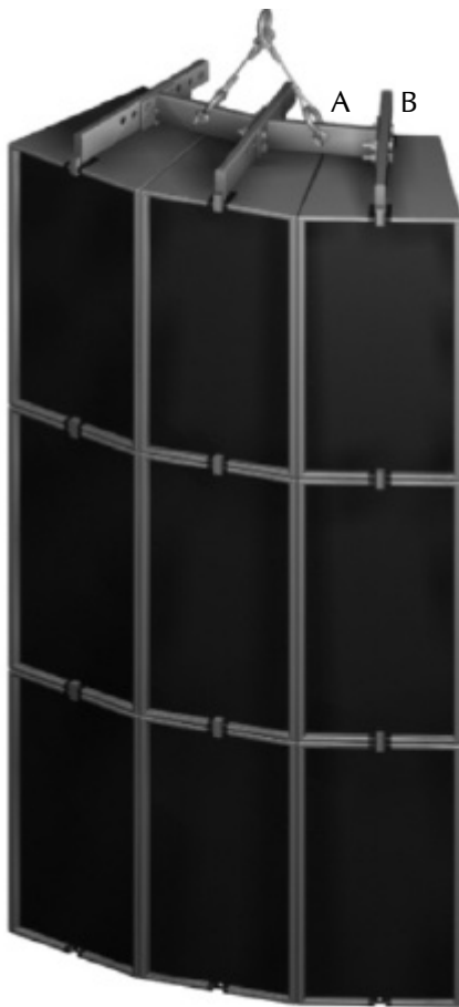
Fig.1 Three Quick-rig™ Flying Frames [B] with Quick-rig™ 18- degrees connecting bars [A] for waved front configuration.
