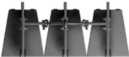
Fig.5 Top view of three arrays with 0-degree frame-to-frame connecting bars.
